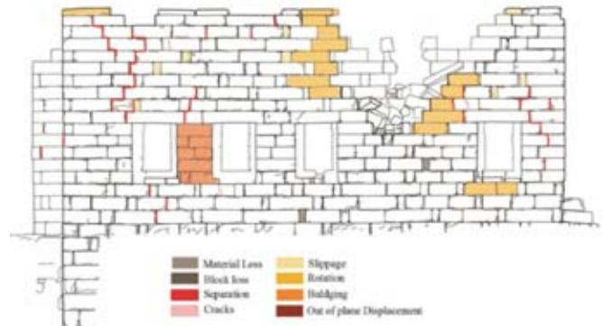
**Fig. 4 : Mapping of structural problems on south facade (© METU, 2012).**
