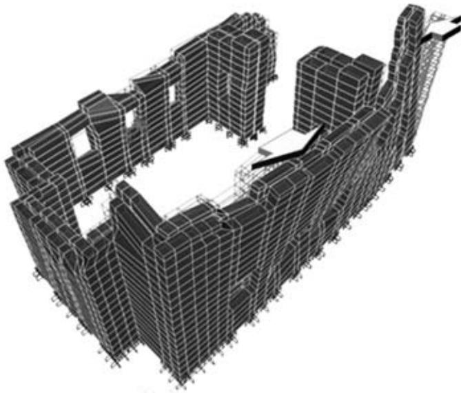
**Fig. 5 : Finite element model of Andron A**
