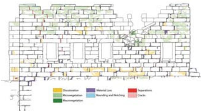
**Fig. 3 : Mapping of visual weathering forms on south facade (© METU, 2012).**
